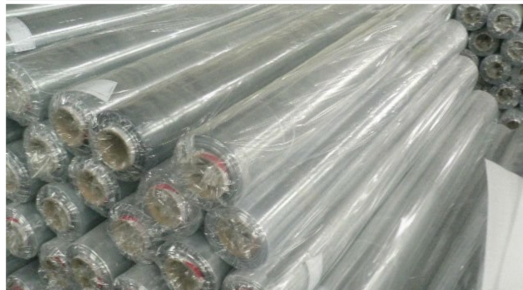
(above) PVC rolls produced by calendaring.
